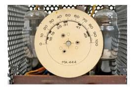
The frequency dial, a piece of printed paper glued onto a disc, was visible through a circular window at the front.
