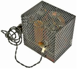
Rear view of the MA 444 Svenkesuperen. Note the headphones sockets at the bottom right. The aerial was connected to a socket at the top.
